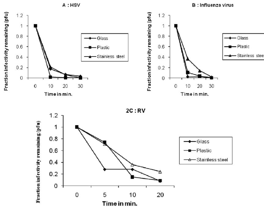
**FIGURE 2.** Kinetics of inactivation of viruses on different surfaces. Multiple aliquots of each virus, in separate experiments in the laboratory, were dried onto the different surfaces, and exposed to ozone gas (10 ppm) at ambient humidity (45% RH). Periodically duplicate samples were removed for reconstitution and freezing. They were subsequently thawed and assayed by plaque formation on the appropriate cell lines.
