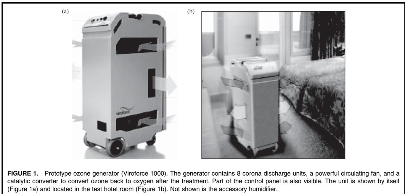
**FIGURE 1.** Prototype ozone generator (Viroforce 1000). The generator contains 8 corona discharge units, a powerful circulating fan, and a catalytic converter to convert ozone back to oxygen after the treatment. Part of the control panel is also visible. The unit is shown by itself (Figure 1a) and located in the test hotel room (Figure 1b). Not shown is the accessory humidifier.
